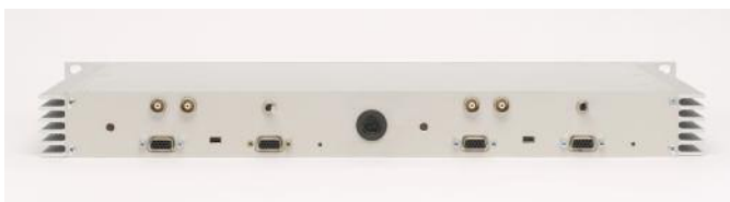
Two channel ultrasonic board from rear side with interfaces and connectors for the PC module and the probes.
